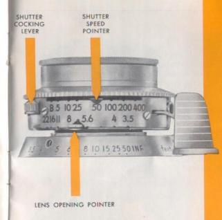
To select the shutter speed, turn the knurled speed control ring until the SHUTTER SPEED POINTER clicks in at the desired speed marking. Do not set the pointer between speed markings.
