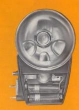
In case you are unable to obtain a 15-volt battery, first remove the B-C Flashpack unit; then insert two 1½-volt penlite batteries in the flasholder with their bases toward the camera side of the flasholder, as shown in the illustration.
